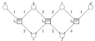
The places are  $P := \{a, b, c, d, e, f\}$  and the polynomials defined by the transitions are  $t_1 := a + b - 2e$ ,  $t_2 := 2b + 2c - e - 2f$  and  $t_3 := c + d - 4f$ . A Gröbner basis (using the order f > e > d > c > b > a) for the ideal generated in  $\mathbb{Q}[P]$  is
