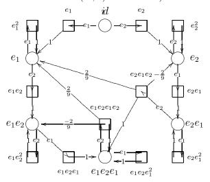
The states of the Petri net are labelled by the irreducible monomials. To reduce a polynomial p take the initial marking  $M_0$  to be such that  $M_0(id) = p$  and  $M_0(m) = 0$  for all other  $m \in P$ . A transition is enabled if the input states to it hold terms which are right multiples of the weight on their input arcs. Firing of a transition transforms the input and all output states simultaneously. For example, if in the
