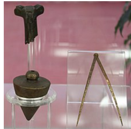
Equipment used by an ancient Roman land surveyor ( gromatici ), found at the site of Aquincum , modern Budapest , Hungary
