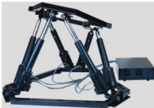
A hexapod consists of two rigid bodies (platform and base), connected by legs. The legs have fixed length and are anchored at platform/base spherical joints.
