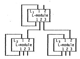
For realizing a data exchange with  $L_3$ ,  $L_1$  has to execute the following instructions: open 1; p:=b; close 1; open 3; a:=p; close 3. By this sequence,  $L_1$  stores the content of cell b in its own memory B to cell a in memory B of  $L_3$ , where p is some variable in the private memory of  $L_1$ . We assume that all switches C initially are closed. The sequence above will be abbreviated by the notation
