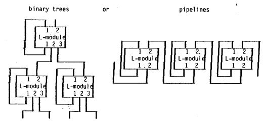
The numbers m and n must be chosen appropriately for the L-modules used for realizing a particular topology. (For example, m=3, n=2 for the binary tree and m=n=2 for the pipeline.) In general, the neighbourhood parameters n and m will be small and so we can construct L-nets of every size and structure.
