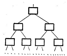
Every node of the tree denotes a (micro-)computer with its own central processing unit and its own storage. The number of nodes in the tree is potentially infinite. (Of course, a practical implementation has to cut off the tree at some level.)
