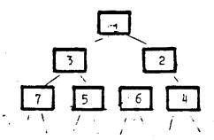
The programs in the modules may be started by a control computer located at the top of the tree similar to Example 4, for instance, by the following intructions:
